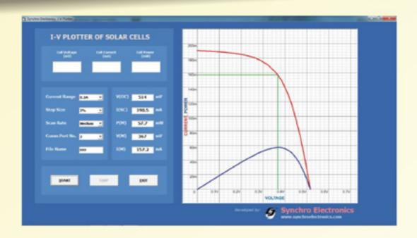
Voltage Range : 1V, 2V, 5V, 10V, 20V, 50V Current Range : 0.2A, 0.5A, 1A, 2A, 5A
